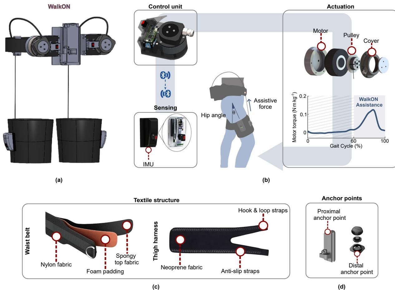
**Extended Data Fig. 2 | WalkON hardware components.** (a) Computer-aided design of WalkON (b) Inertial Measurement Unit (IMU) sensors stream hip motion data via Bluetooth Low Energy to the control unit. This unit runs the control algorithm on a microcontroller. The output is a velocity command sent to
