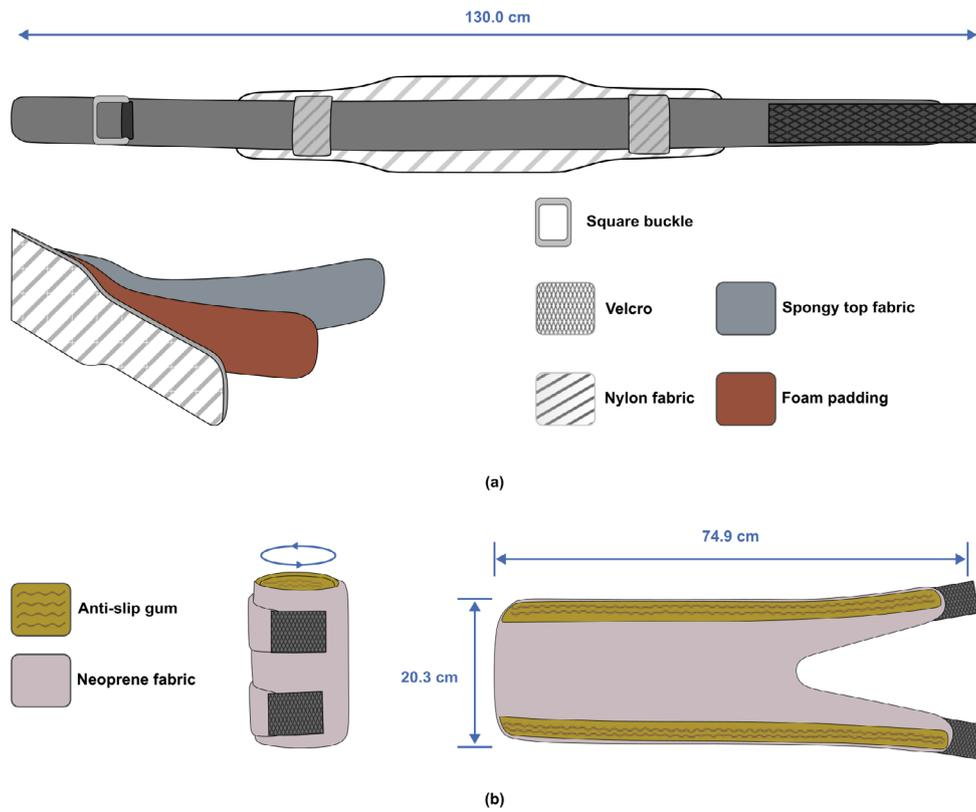
**Extended Data Fig. 1 | Textile blueprint.** (a) WalkON waist belt and layers composition. (b) Thigh textile harness inner view and closed configuration.
