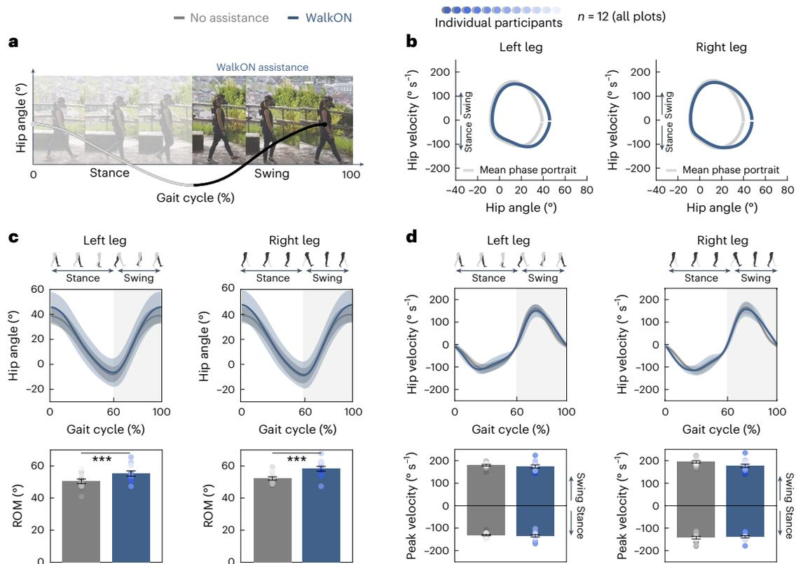
**Fig. 3 | Hip joint motion results for young adults.** **a**, WalkON actively assists the hip joint during swing. **b**, Raw hip phase portraits averaged across steps and subjects, combining hip angle and velocity measured on the sagittal plane. **c**, The hip range of motion (ROM) exhibited a significant increase with WalkON (navy) compared with the no assistance condition (grey). **d**, There were no significant
