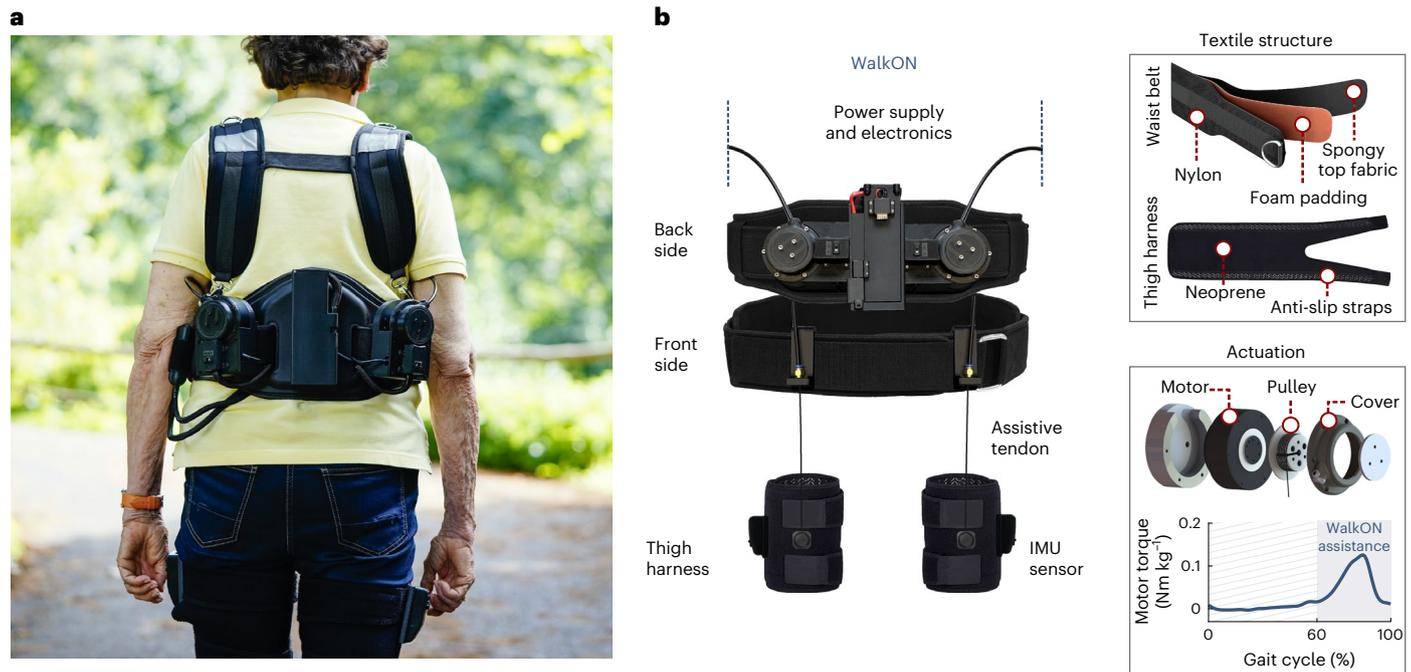
**Fig. 1 | WalkON design.** **a**, An older adult using WalkON for outdoor walking. Photography by Uwe Anspach. **b**, WalkON's design comprises a textile structure encompassing a waist belt and two thigh harnesses that can be comfortably worn over regular clothing. The actuation mechanism relies on a tendon-driven transmission, with artificial tendons linked to the front part of the user's legs.
